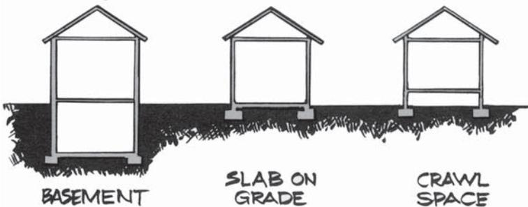
Radon reduction systems can be grouped by house foundation design. Find your type of foundation design above and read about which radon reduction systems may be best for your house.
